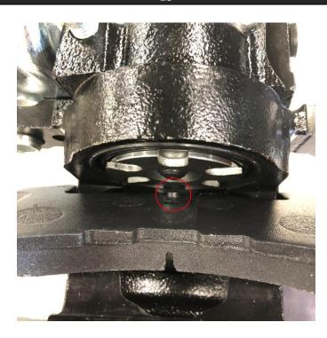
**Kits with parking brake calipers** should be checked to confirm the pad is seated flat against the piston face, with the boss of the brake pad lining up with the notch in the piston face
