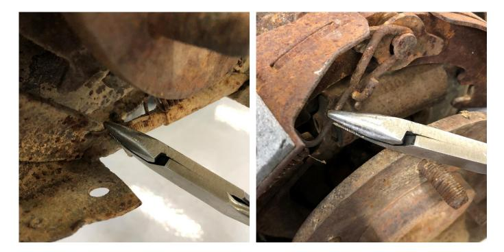
Remove the additional retaining springs from the brake shoes.
